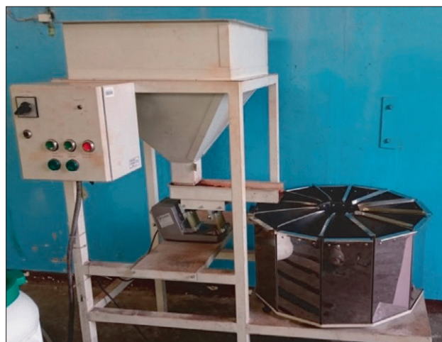
Fig. 1. Twelve-position separator for powder materials used to homogenise of the materials
